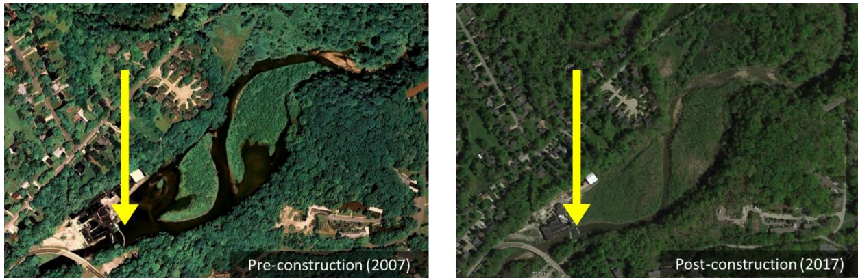
Figure 7. Pre-construction (2007) and post-construction (2017) aerial imagery of the Ives of Ohio lower dam modification and stream restoration project. A yellow arrow indicates the location of the modified dam. Image source: Google Earth.
