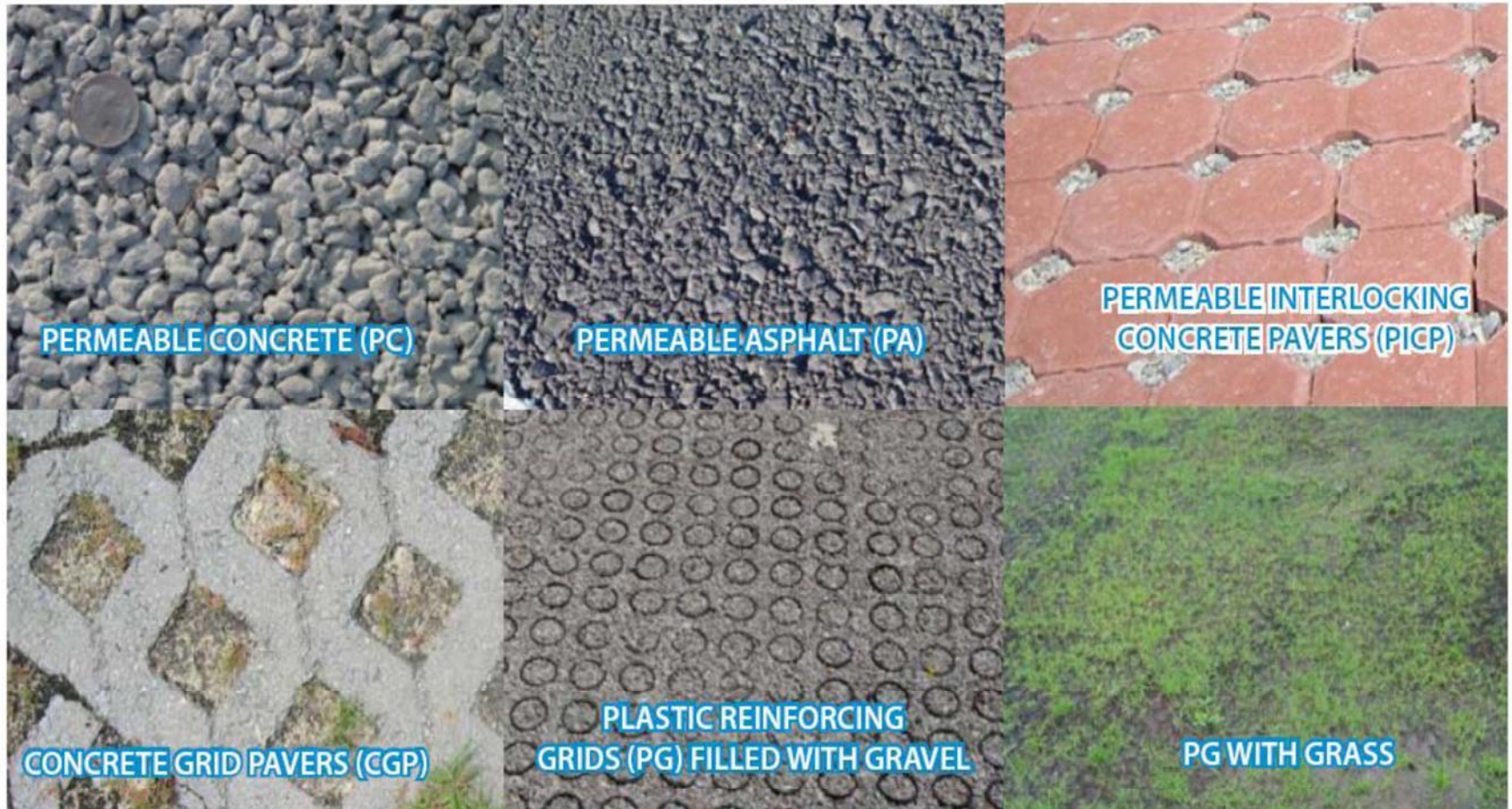
Figure 2. Types of permeable pavement
