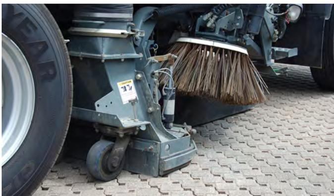
Vacuum sweeper trucks can be used for permeable pavements
