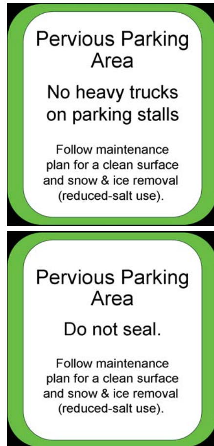
Figure 2.11.13 Examples of signage that might be used to protect pervious pavements.
