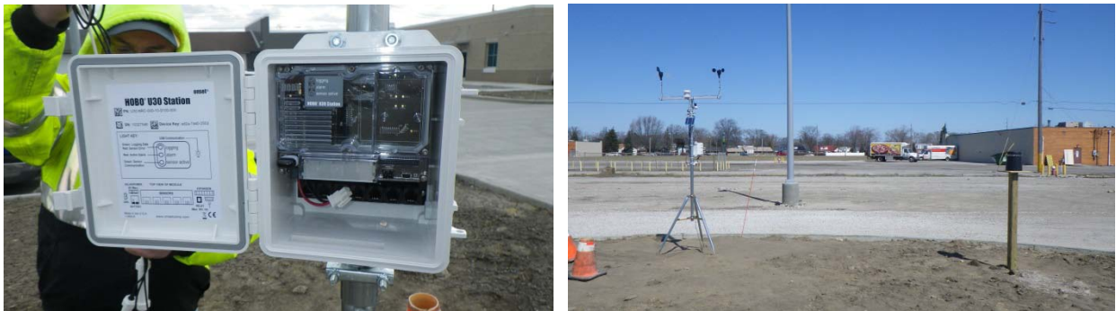
Figure 9. Hobo U30 data logger attached to weather station mast (left). Photo of rain gauge and weather station located at Perkins Township (right).
