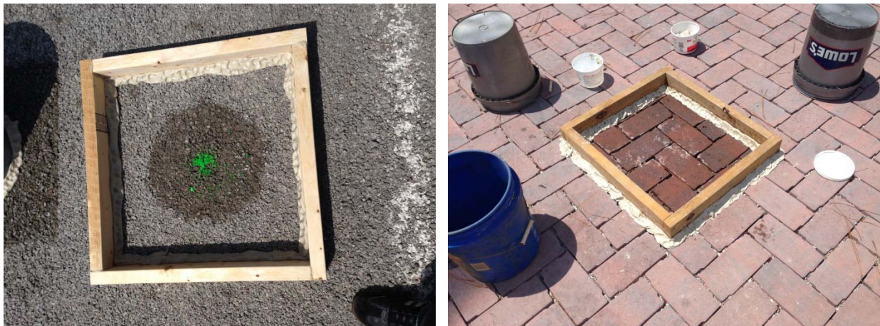
Figure 65. Surface infiltration rate testing using the SIT method on PC (left) and PICP (right).
