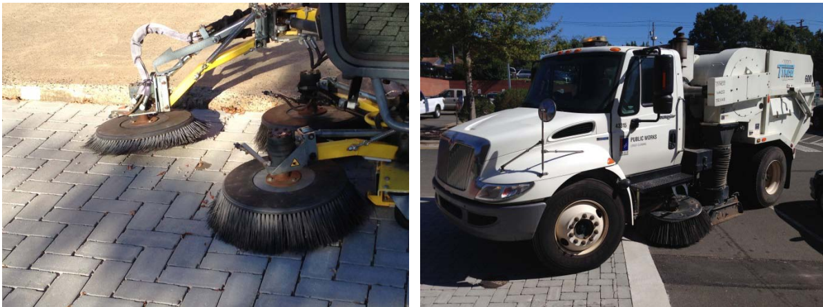
Figure 75. Standard bristle street sweeper (left) and regenerative air street sweeper (right) performing maintenance at NCCU.
