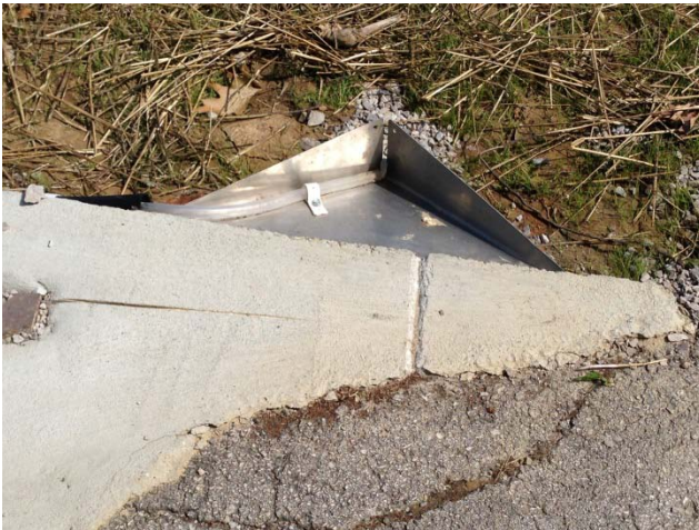
Figure 44. Sampling trough with sample intake to sample runoff quality from the asphalt pavement (left) and the spigot from which water quality samples were obtained to characterize the quality of the water at the point-of-use (right) at Old Woman Creek NERR.
