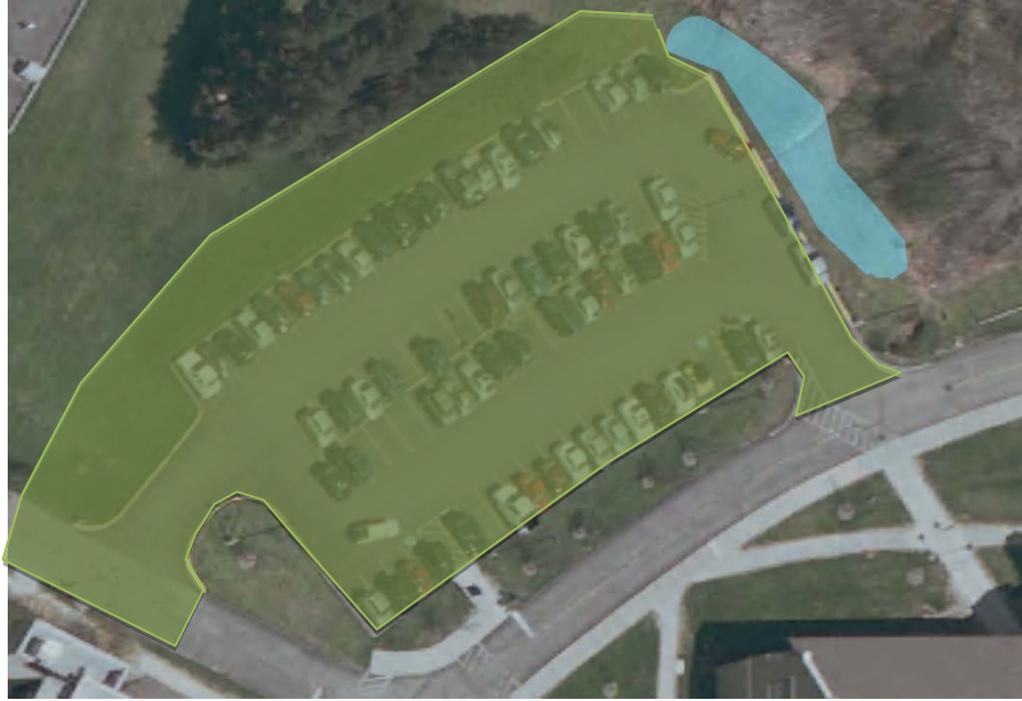
Figure 21. Watershed overview for the Ursuline College bioretention cell site. The watershed is outlined in green and the bioretention cell in blue.
