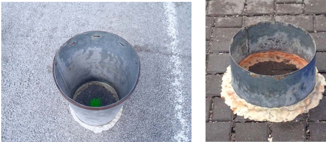
Figure 64. ASTM surface infiltration rate tests on PC (left) and PICP (right).
