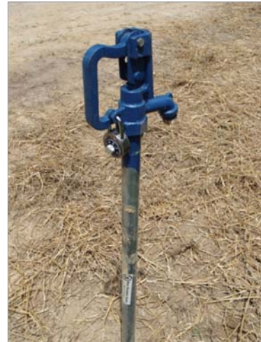
Figure 44. Sampling trough with sample intake to sample runoff quality from the asphalt pavement (left) and the spigot from which water quality samples were obtained to characterize the quality of the water at the point-of-use (right) at Old Woman Creek NERR.
