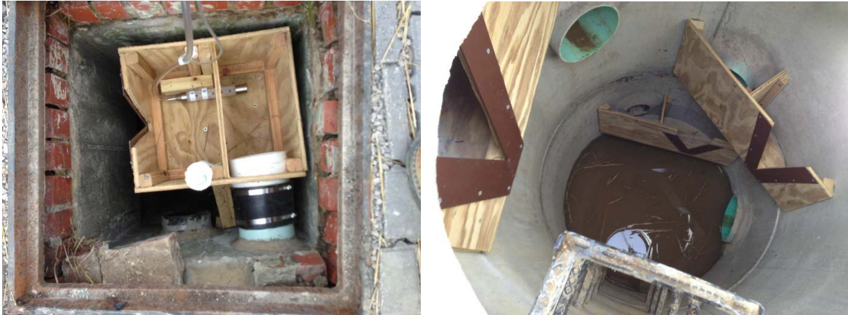
Figure 10. Weir boxes at Willoughby Hills Small application (left) and Orange Village (right). Note 6” underdrain tying into weir box at left. Note presence of three weir boxes at right. The upper weir box is connected to the underdrain for the permeable pavement, while the middle and lower ones measure drainage from the bioretention cell and the curtain drains at Orange Village.
