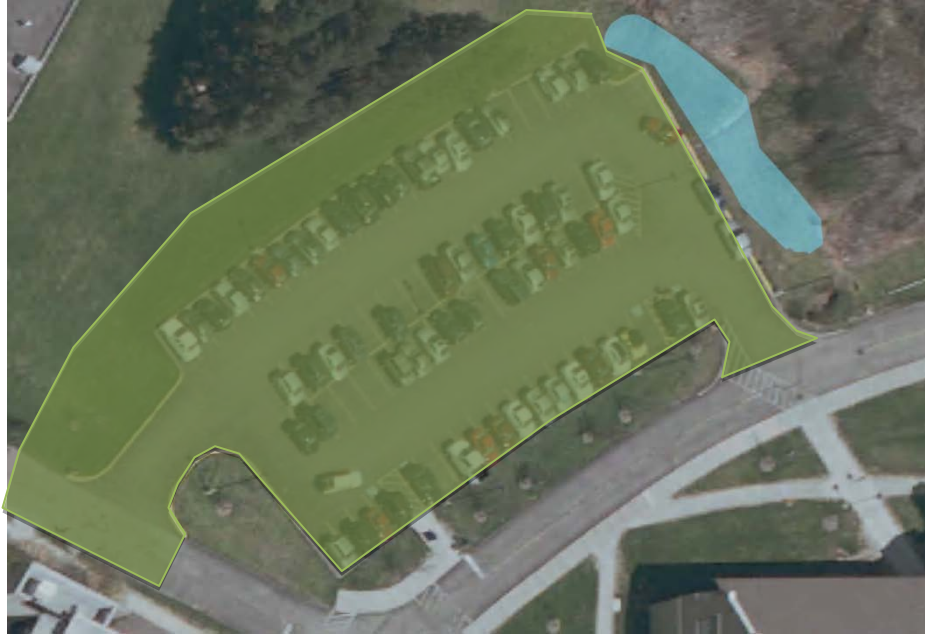
Figure 52. Watershed overview for the Ursuline College bioretention cell site. The watershed is outlined in green and the bioretention cell in blue.
