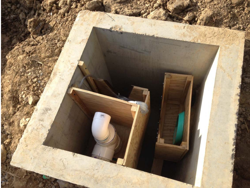
Figure 45. Weirs for drainage (at left) and overflow (at right) measurement in the monitoring vault at Old Woman Creek NERR.
