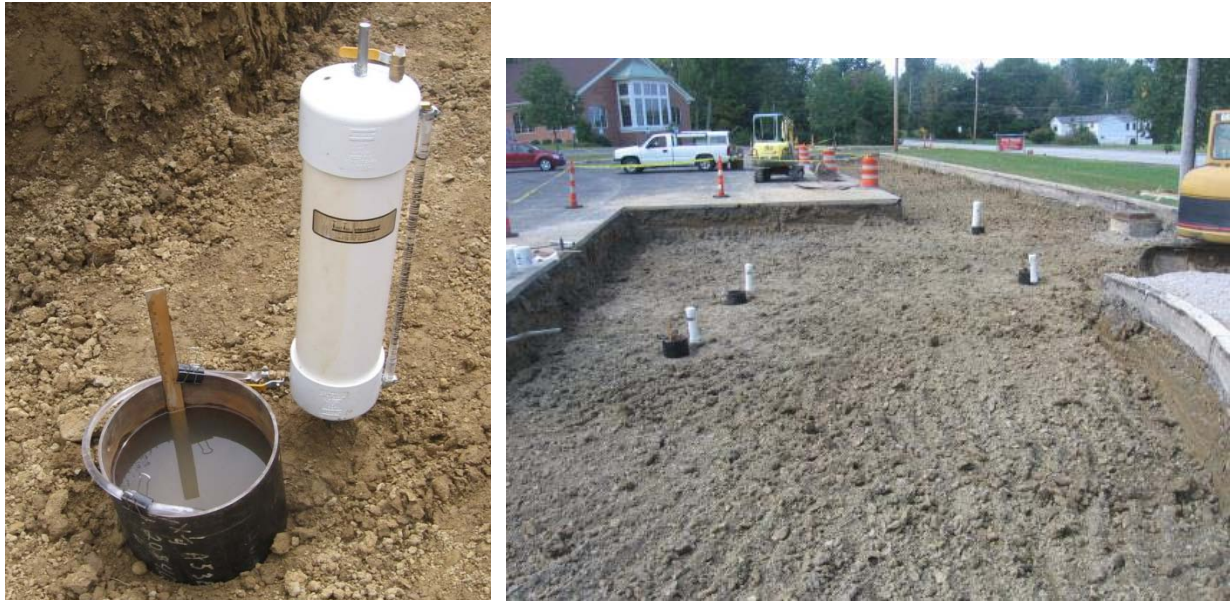
Figure 11. Single ring, constant head hydraulic conductivity test with Mariotte syphon (left) and hydraulic conductivity tests being carried out at the Willoughby Hills Large application (right).
