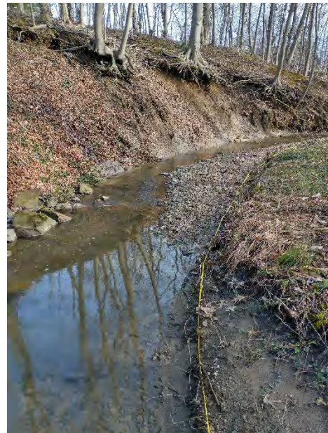
Figure 3. Streambank in Pepper Pike with a BEHI rating of "very high."
